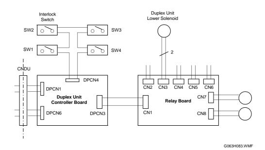
Defective duplex unit lower solenoid. Defective duplex unit controller board.
