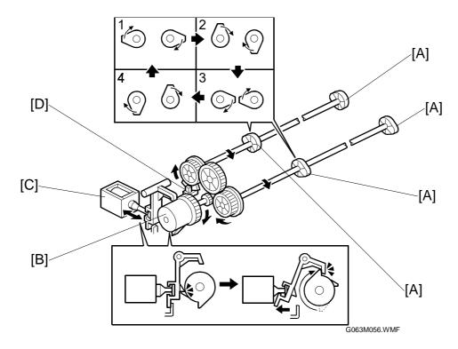
When the printer is idle, none of the toner cartridges contacts the OPC belt. During printing, the machine moves the toner cartridges into contact with the belt one at a time, in the order K, C, M, Y.
