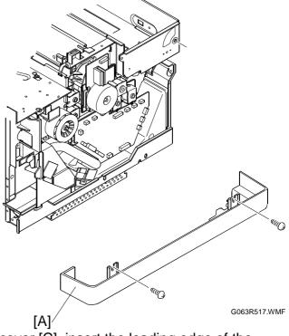
**NOTE:** 1) When assembling the base cover [C], insert the leading edge of the base cover over the hooks [B] (2 locations) provided at the bottom (left and right) of the base plate [C].
