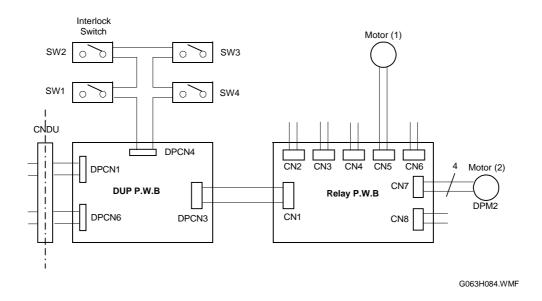
Defective duplex unit motor (1) or (2).
