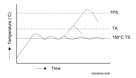
TS: The machine maintains a temperature of about 150°C by turning the thyristor on/off.
