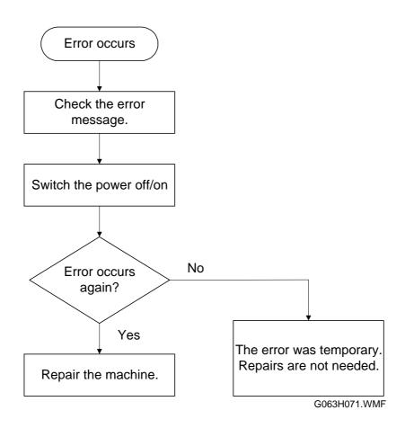
If a printer engine error occurs, the operation panel will display an error message, and the printer will stop. If the error occurs again after the machine is switched off/on, repair the machine. The rest of this section contains guidelines on how to repair the machine for each error code.
