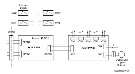
Defective duplex unit upper solenoid. Defective duplex unit controller board.
