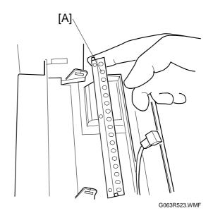
**NOTE:** Do not touch the transfer drum with your bare hands while removing or reassembling the erase lamp.
