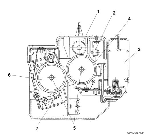
1. Cleaning Roller Cleans the hot roller.
