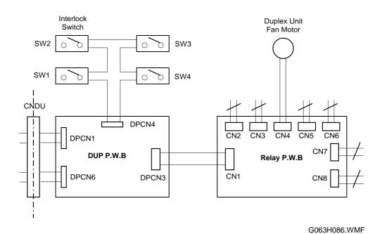
Defective duplex unit fan motor. Defective duplex unit controller board. 17 January, 2001 IMAGING FAILURE
